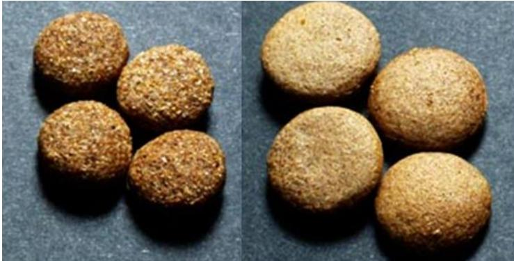
Photo 3: Difference in finer grinding, product on right looks better and is of lighter density. Finer grinding give versatility in running for desired densities.
