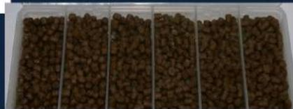
Photo 2: Pellets coated and uncoated, cell structure example for high oil uptake and various density raw pellets with correct cell structure can pick up various oil levels and all be sinking densities.
