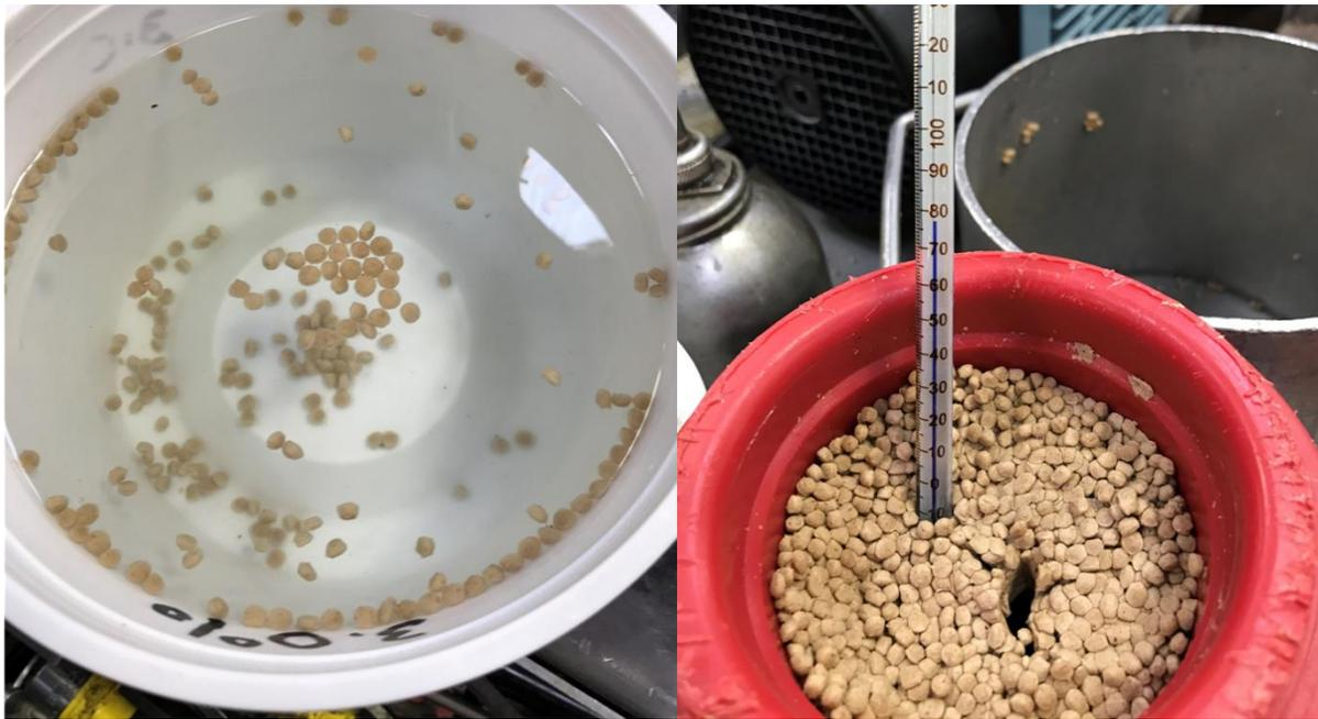
Photo 6: Neutral Buoyant Feed test 3% salt water and products made at less than 80°C.
